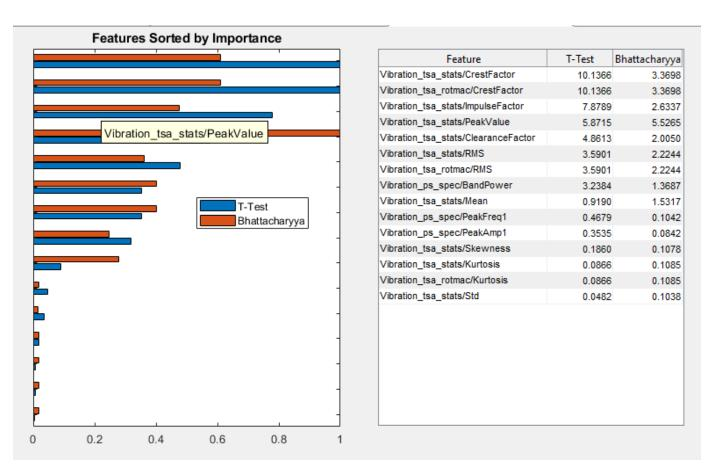
The Bhattacharyya technique yields results that are similar to, but not identical to, the T-Test results. The highest ranking feature is PeakValue from the Signal Statistics set.
