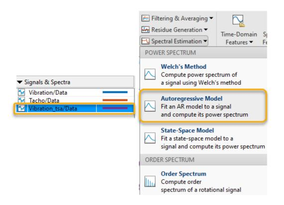
The **Autoregressive Model** tab provides parameters that you can modify. Accept the default values by clicking **Apply**.
