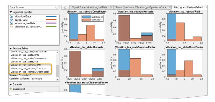
The app automatically adds the new features to the feature table and the **Select Features** list, and plots the new histograms at the top of the histogram display. CrestFactor and Kurtosis histograms are essentially the same whether they were computed as signal features or rotating machinery features, since both computations used the TSA signal as a source.
