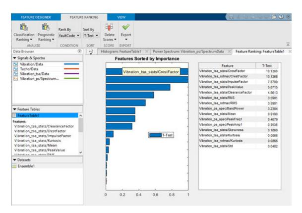
The bar chart legend shows that the initial ranking is performed using the T-Test algorithm. The chart is normalized to 1 to facilitate visual comparison. The table displays unnormalized ranking scores. Hover your mouse over a bar to get the full variable name.
