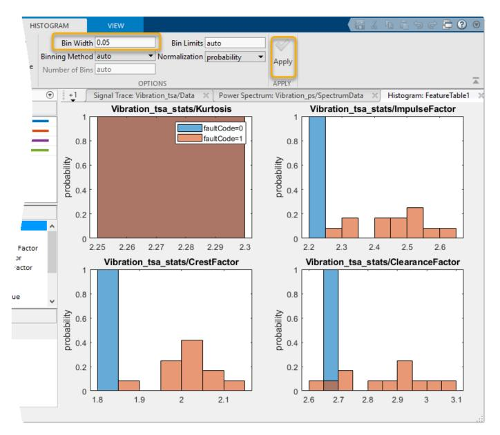
At this resolution, both CrestFactor and ImpulseFactor appear to completely separate healthy from faulty data. ClearanceFactor still has some mixed data, but to a lesser degree than with the larger bin width. Kurtosis had a smaller bin width of 0.002 with the auto bin width setting. Changing the bin width to 0.05 results in a single bin that contains all the Kurtosis data.
