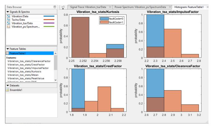
Control the appearance of the histograms using the parameters in the **Histogram** tab, which activates when you generate the histograms. The CrestFactor feature appears to separate healthy and unhealthy data almost completely. Investigate whether this result is sensitive to resolution. In the **Histogram** tab, the auto setting of bin width results in a resolution of 0.1 for CrestFactor. Enter a bin width 0.05, and click **Apply**.
